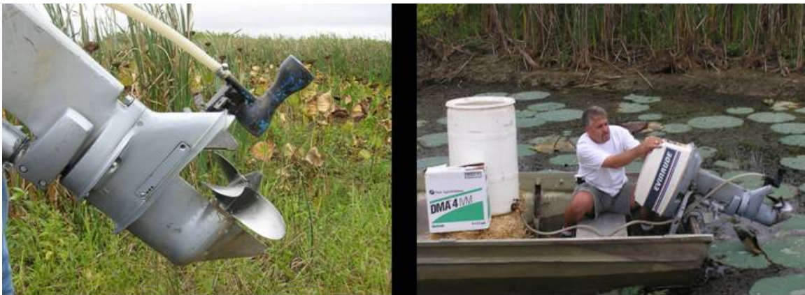
Figure 4. Boat bailer system used to distribute herbicide.
